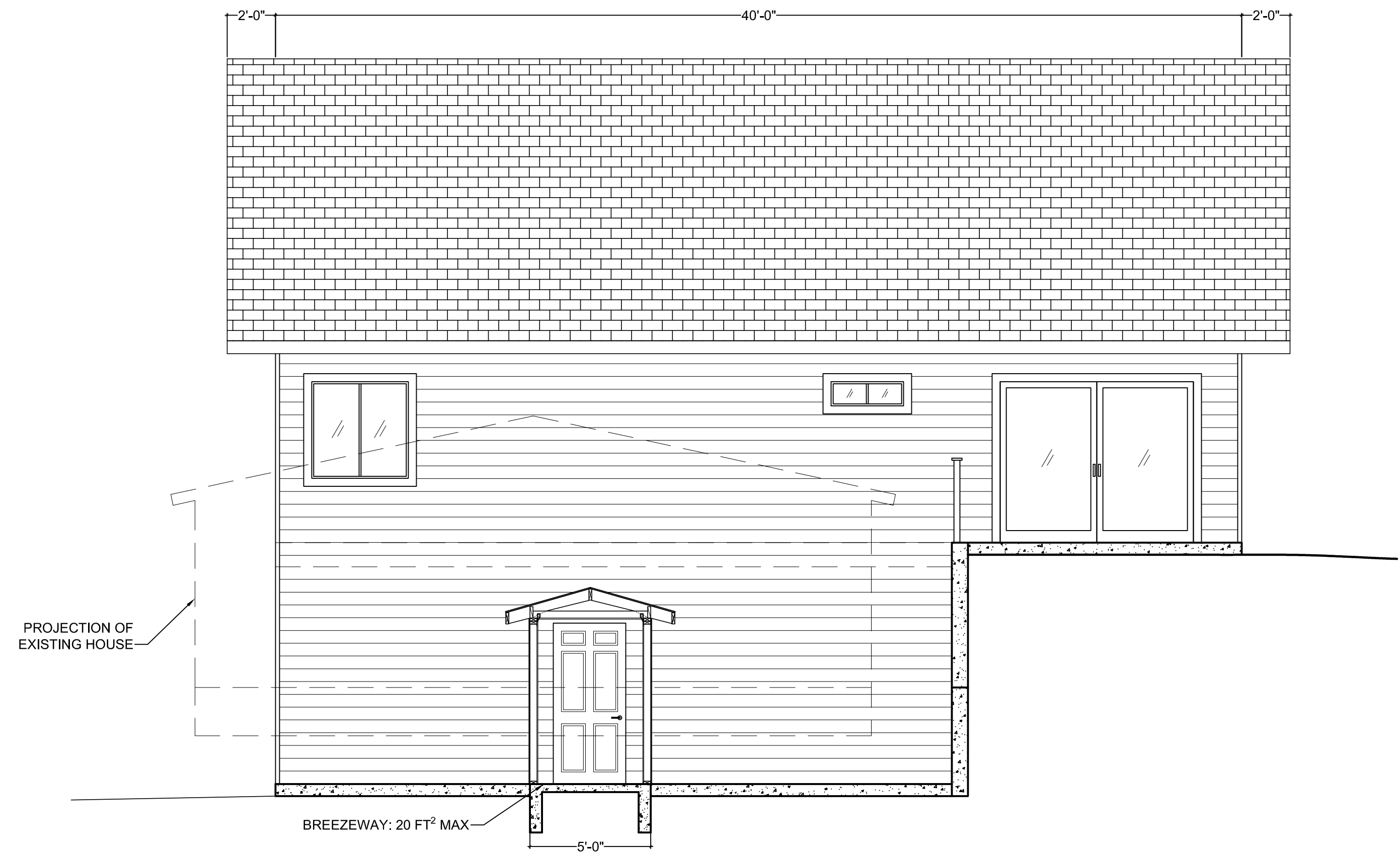
B-3 A1.1 NEW STRUCTURE, EAST ELEVATION SCALE: 1/4" = 1'-0"
